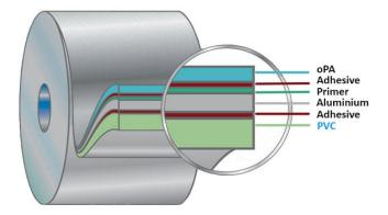
The Alu-Alu foil can be shaped in various appearances by changing the mould. The most common structure used in these foil laminates are 25µ OPA/Adhesive/45µ Aluminum Foil/Adhesive/60µ PVC.
