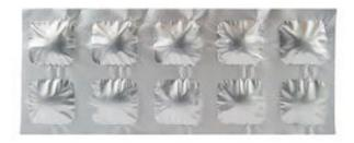
We have different gauges with most common being  $25\mu/30\mu/40\mu$  for pharmaceutical applications. The foils have LDPE Laminated on one side having standard polymer gaueg 150/180/200 with tolerance level of +/- 15% confirming to the applicable government regulations regarding the direct contact with drugs and medicines & other side is plain or printed as per customer needs.
